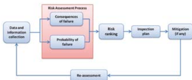
Figure 3: Risk-based inspection planning process [4]
